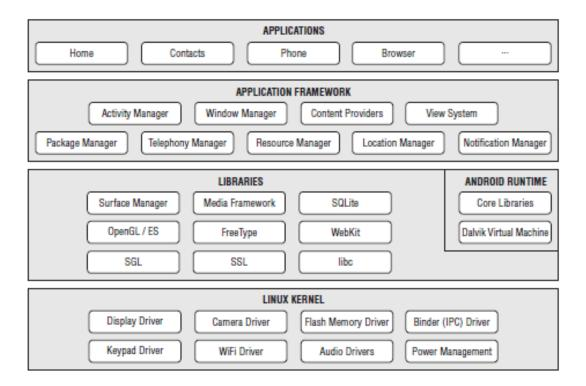
The Android OS is roughly divided into five sections in four main layers:
